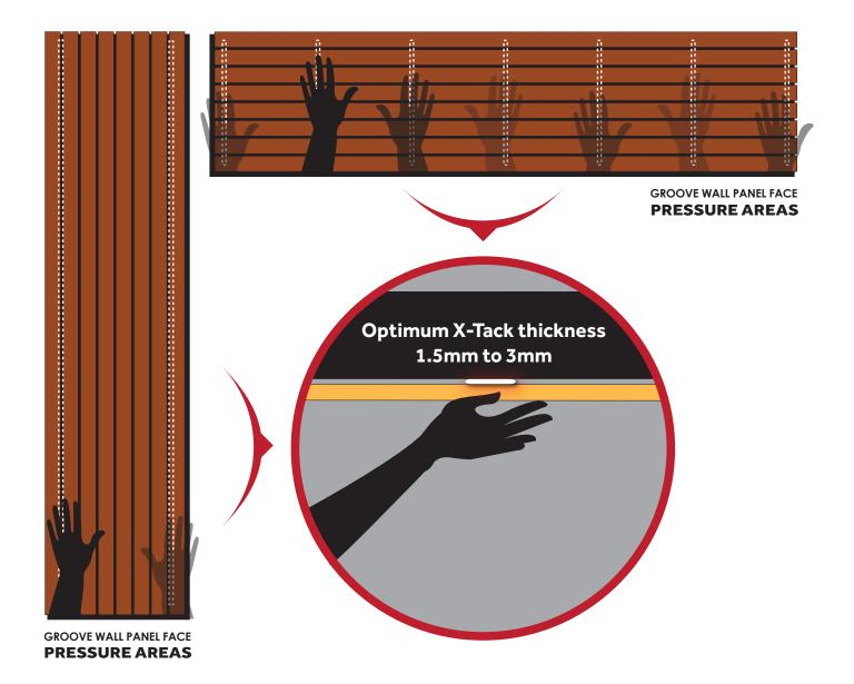
Be sure to have surfaces bonded within five minutes from commencing X-Tack application. Once the panel has been pushed firmly into position, the optimum thickness for X-Tack is 1.5mm - 3mm.
